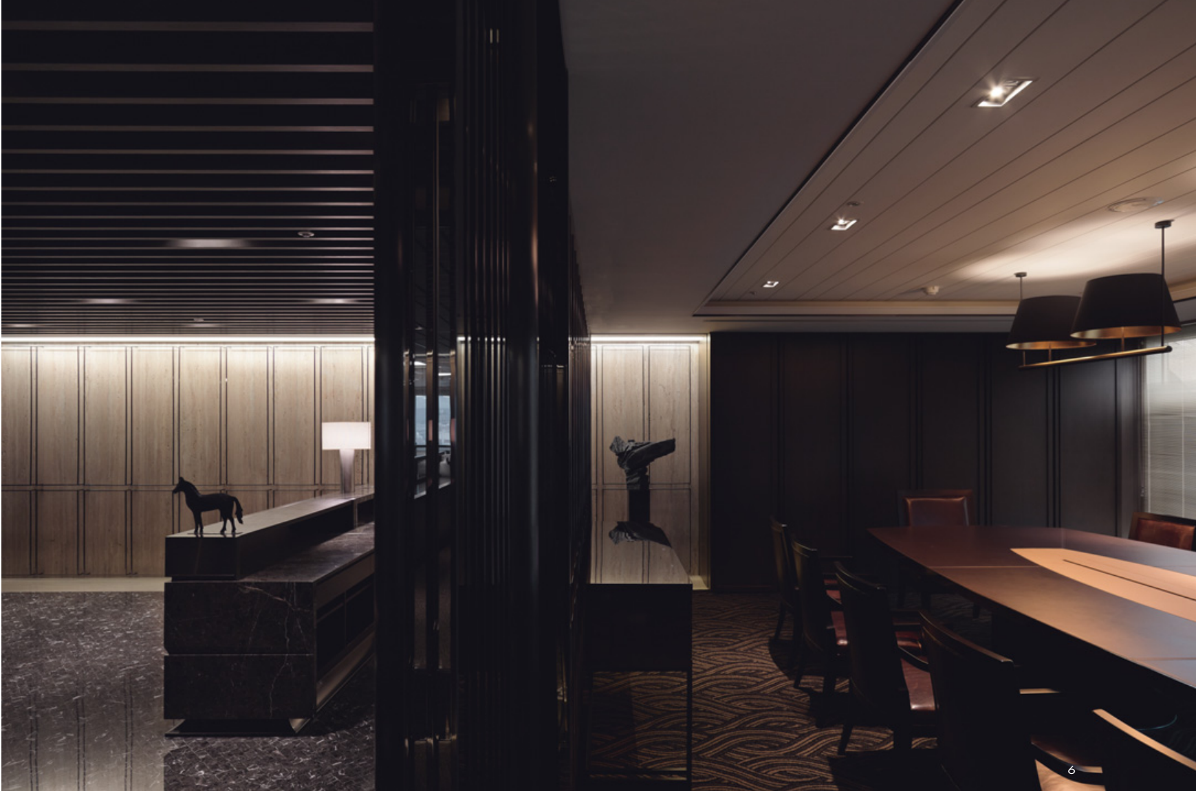
6. 接待大廳與會議室間以金屬格柵門片銜接。7. 會議室視訊立面以義大利櫟木分割拼貼結合鍍鈦板及45度倒角分割縫處理。8. 會議室正立面以玫瑰金鍍鈦板做幾何分割，底層為鐵刀木和皮革。9. 自接待大廳望向會議室，藉由實相映的格柵或玻璃，賦予空間趣味性。 6. Grating metal door linking reception and conference room 7. The surface treatment in the conference room reveals Italian black wood patterned with metal panels 8. Conference room and its surface treatment in metal, hardwood and leather detailing 9. Vista view from reception towards the conference room
