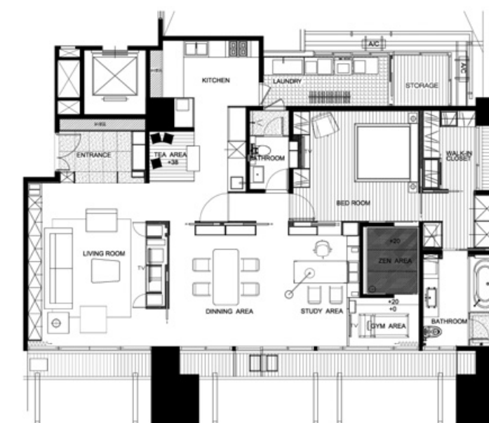
3. 所有作為界定空間的牆，像是脫離外牆般，獨立存在著。4. 平面配置圖。 3. Partition in this apartment is detached structurally from the actual load bearing system 4. Plan
